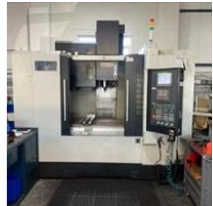
3: XYZ SM SLV3000 CNC Milling Machine with ProtoTrak SM Control. Retrofitted with New Control 2023
