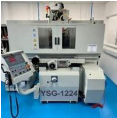
1: ANDMAR Model YSG-1224 TS CNC Precision Hydraulic Surface Grinder. Year 2022
